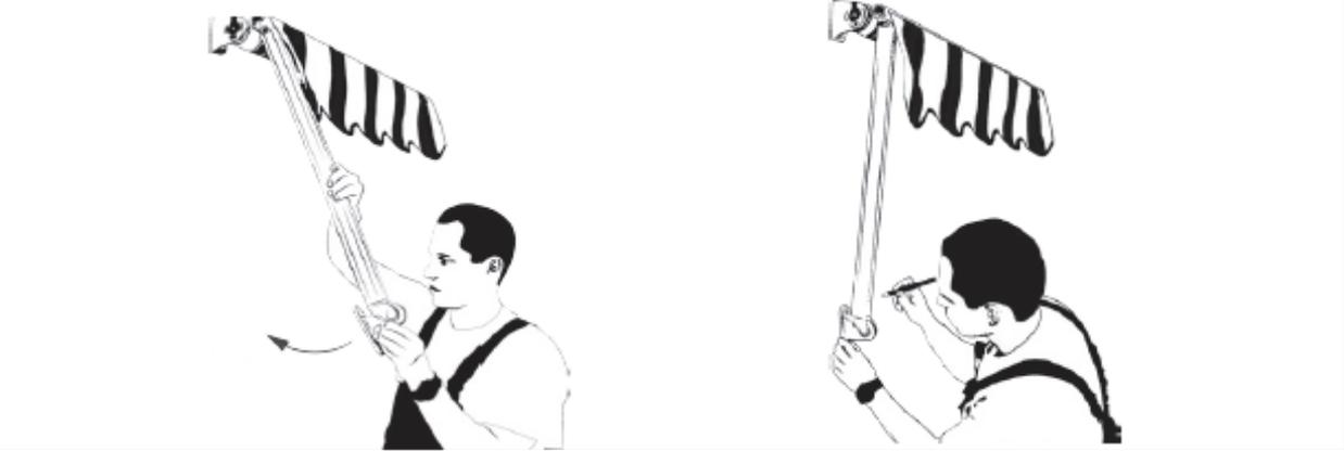
19) Unscrew the arm from the front bar and drill holes in marked places.
